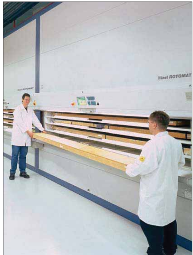
Secure storage of bulky parts in the Rotomat® industrial carousel
